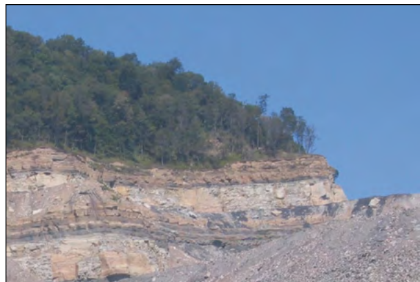
Figure 3-10.—Weathered overburden above unweathered materials. Weathered overburden can be found immediately below the soil and often extends to about 30 feet beneath the surface—although it may be deeper. The weathered overburden, which has been affected by surface processes, is better material to place on the surface for forestry land uses than unweathered gray materials. Photo by C. Zipper, Virginia Tech, used with permission.
