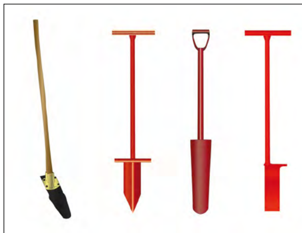
Figure 9-4.—Tree-planting tools commonly used on mine sites. From left to right: hoedad, KBC planting bar, sharpshooter spade, and dibble bar.
