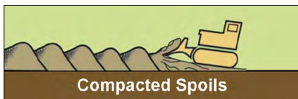
Figure 4-5.—Diagram illustrating the “dozer push-up” method. This method can be used to prepare uncompacted surfaces that are suitable for reforestation where materials for surface placement are moved over a short distance. Depending on the situation and State program policies, it may be possible to use the “dozer push-up” surface for reforestation without a final strike-off grading. Otherwise, the push-up piles should be struck off with one or, at most, two passes with a light dozer.
