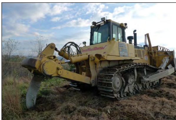
Figure 10-4.—Ripping tooth on the back of a dozer. The ripping tooth can be inserted into and pulled through the ground to loosen the dense mine soil, improving its physical properties and ability to support planted trees. Photo by N. Hall, Green Forests Work, used with permission.
