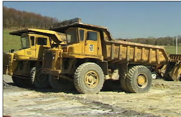
Figure 5-1.—Haul trucks, which can weigh 50 to 100 tons or more even when empty. This weight exerts force where tires meet the land surface, causing severe compaction of mine soils. When operated on surface soils, loaders, dozers, and other heavy mining equipment also cause compaction that hinders tree growth. Photo by J. Skousen, West Virginia University, used with permission.
