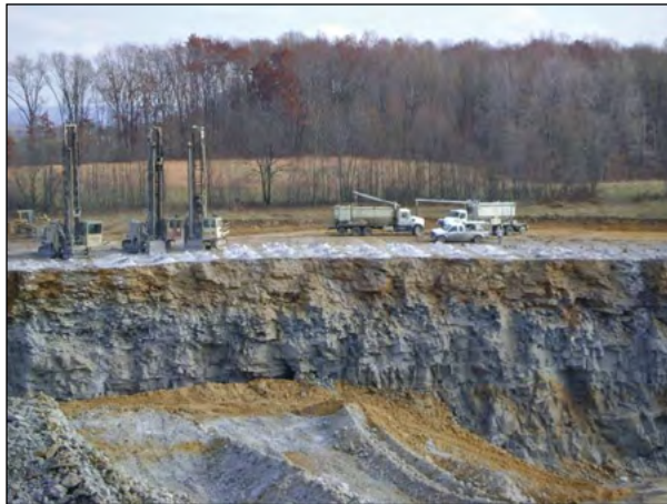
Figure 3-3.—Overburden consisting of weathered brown sandstone over unweathered gray sandstone and siltstone. The native soil has been stripped off the surface before blasting and mining. A native plant community is growing on native soils in the background. Photo by J. Skousen, West Virginia University, used with permission.
