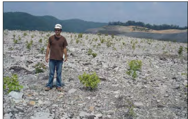
Figure 3-5.—Unweathered gray sandstone on the same West Virginia mine site as in Figure 3-4 after 2 years showing some weathering into smaller particles, but generally poor tree growth and poor colonization by native plants. The pH is above 8.0. Photo by J. Skousen, West Virginia University, used with permission.
