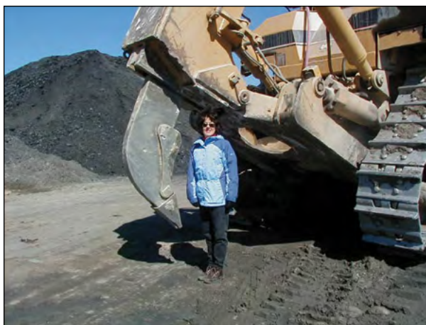
Figure 5-3.—A single-shank ripper attached to a dozer. This type of ripper is capable of ripping the soil to a depth suitable for forest trees when attached to a large dozer. Photo by P. Angel, OSMRE.
