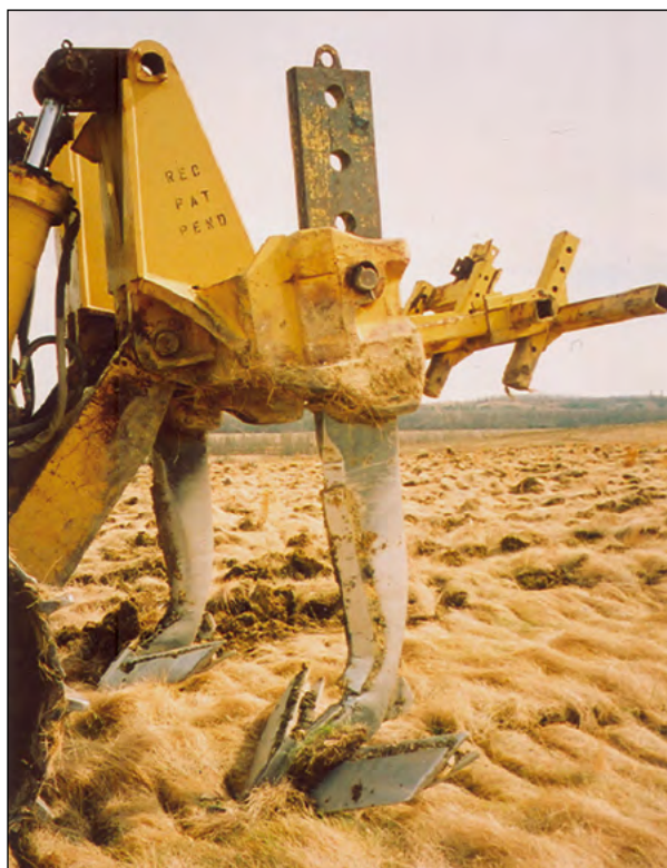
Figure 5-5.—A ripper with a plow attachment, which can be used to loosen soils that do not contain large rocks and boulders. The "wings" on the ripper blades will loosen soils located next to the ripping trench. Photo by D. Graves, University of Kentucky, used with permission.
